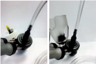
With a bottle mount tubing combination it is recommended to partially prime the tubing side first, than afterwards the bottle mount side. This will avoid product waste on the bottle mount side during the priming of the tubing.
